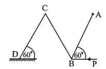
The system is kept in equilibrium with the rods making an angle  $\frac{\pi}{3}$  to the horizontal by a horizontal force P applied at B. If the coefficient of friction between the surfaces at D is  $\mu$ , show that  $\mu \geq \frac{\sqrt{3}}{7}$ . Find the horizontal and vertical components of the reaction exerted by BC on DC at C. Also show that  $P = \frac{5w}{2\sqrt{3}}$ .
