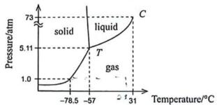
It is observed that liquid CO<sub>2</sub> does not form when a sample of solid CO<sub>2</sub> (dry-ice) is placed in a beaker at 25 °C and 1 atm pressure. According to the above diagram which of the following statement/s explain/s this observation?
