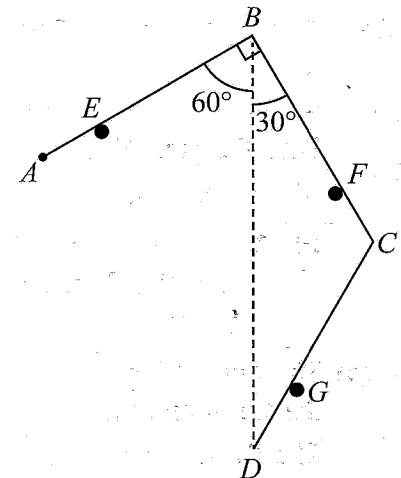
(b) The framework shown in the figure consists of five light rods  $AB$ ,  $BC$ ,  $CA$ ,  $CD$  and  $DB$  that are smoothly jointed at their ends. It is given that  $AB = BC = CA = 2a$ ,  $\hat{CBD} = 90^\circ$  and  $\hat{BCD} = 60^\circ$ . A load  $W$  is suspended at the joint  $D$  and the framework is smoothly hinged to a fixed point at  $A$  and kept in equilibrium in a vertical plane with  $AB$  horizontal, by a force  $P$  applied vertically upwards to it at the joint  $B$ .
