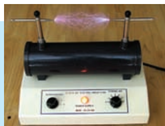
Figure 17.6 - Producing sparks by the induction coil
