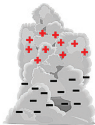
Figure 17.3 - How charges are distributed in a cumulonimbus cloud
