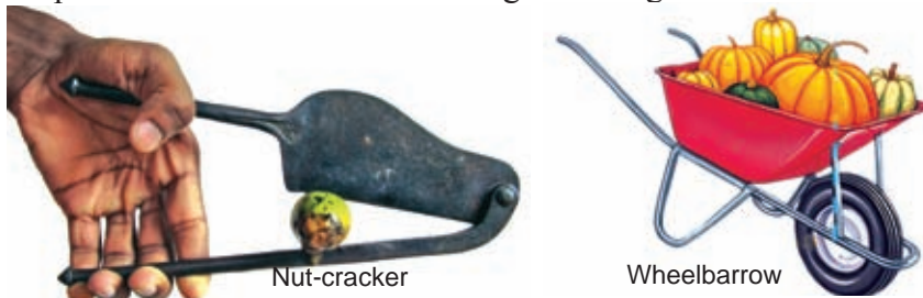
Figure 15.13 – Second order levers
