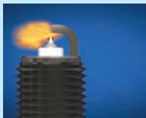
Figure 17.7 - Sparking in a spark plug
