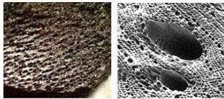
Figure 2: Activated carbon structure - SEM pictures.
