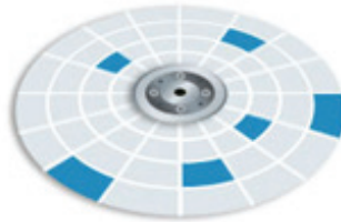
Figure 5.16 - How a file is stored in different places of a disk
