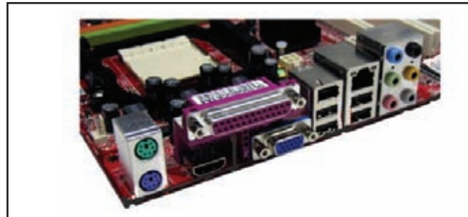
Figure 2.49 - How ports are connected to the Motherboard
