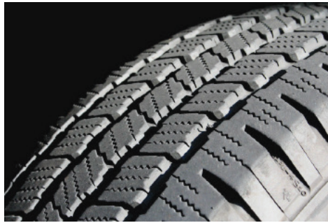
Figure 5.7 – Tires with grooves to increase friction
