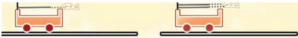
Figure 4.6 - Demonstrating that the acceleration of a trolley increases with force
