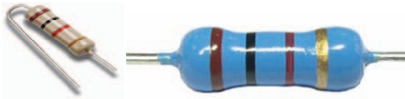
Figure 19.25 – Resistor values marked on the body of resistors using the color code method
