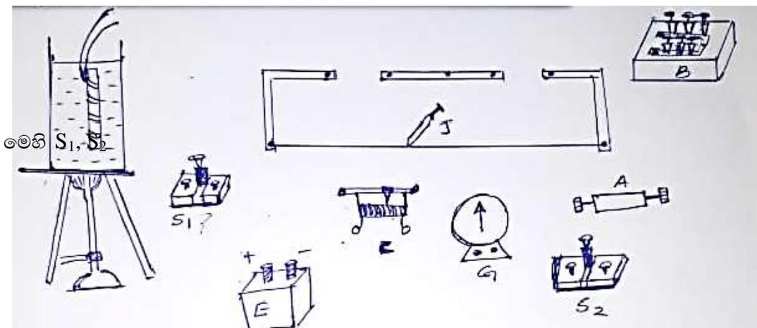
E, a plug switch, Lead acid accumulater a, centre zero Galvanometer, J, (Jockey) sliding key. A is a large resistance. B and C are resistance box and variable resistor respectively.
