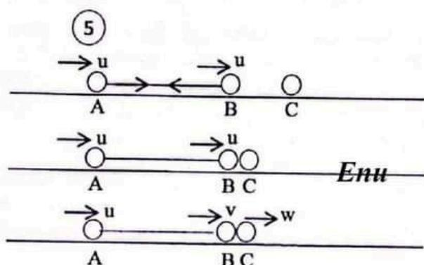
$$\begin{aligned} \text{කාල } &\rightarrow v_1 \rightarrow v_2 \\ \text{විටු } &\quad \text{A} \quad \text{B} \\ \text{විටු } &\rightarrow v_1 \rightarrow v_2 \\ v_2 - v_1 &= e(u_1 - u_2) \end{aligned}$$
