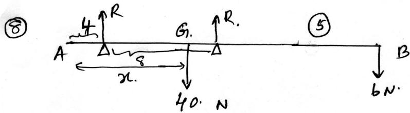
$$\begin{aligned} \uparrow 2R - 40 - 6 &= 0 \quad (5) \\ R &= 23 \text{ N.} \quad (5) \end{aligned}$$
