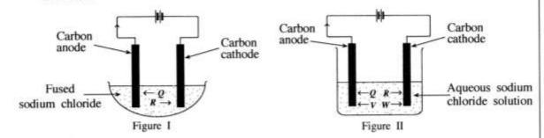
The ions Q, R, V and W move in the directions indicated by the arrows during electrolysis. Of these the ions Q and R are common to both cells.
