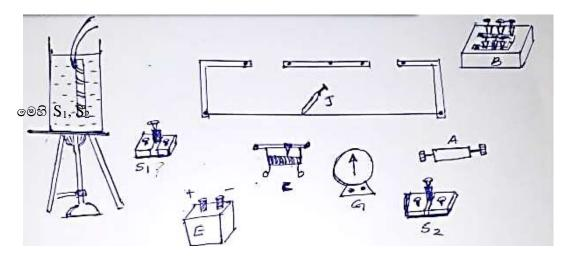
E, a plug switch, Lead acid accumilater a, centre zero Galvanometer, J, (Jockey) sliding key. A is a large resistance. B and C are resistence box and variable resistor respectively.
